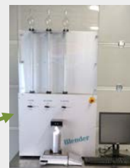
Fuels transfer from main drums directly to Blender back input
